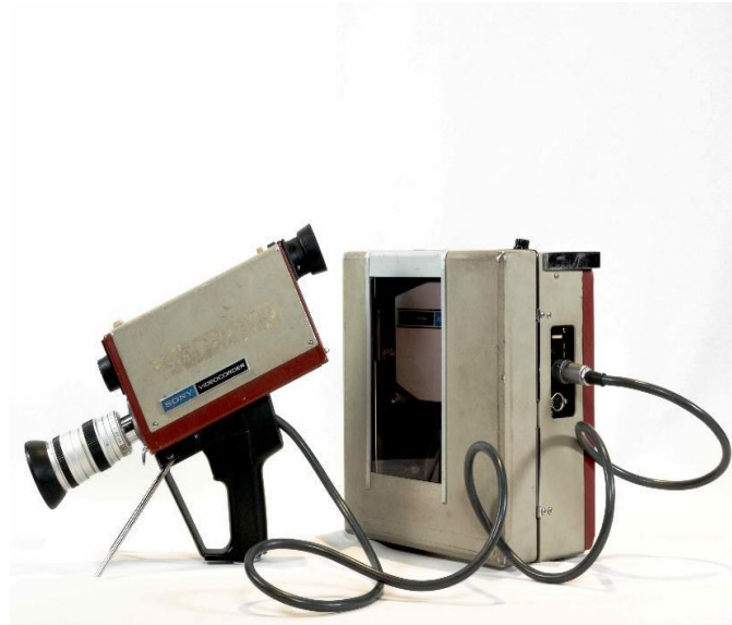
Sony Portapak Video Rover II AV-3400 1/2-in. Camera and Recorder Cinémathèque québécoise collection 1993.0395.01-03. AP TECHNÈS CC BY-SA 4.0
